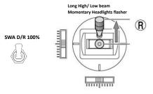
To turn the hazard lights on/off, use the horizontal left stick to the left long with D/R 75%.
