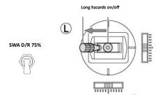
For signals indicators on/off, use the horizontal left stick to the left or right momentary with D/R 100%.
